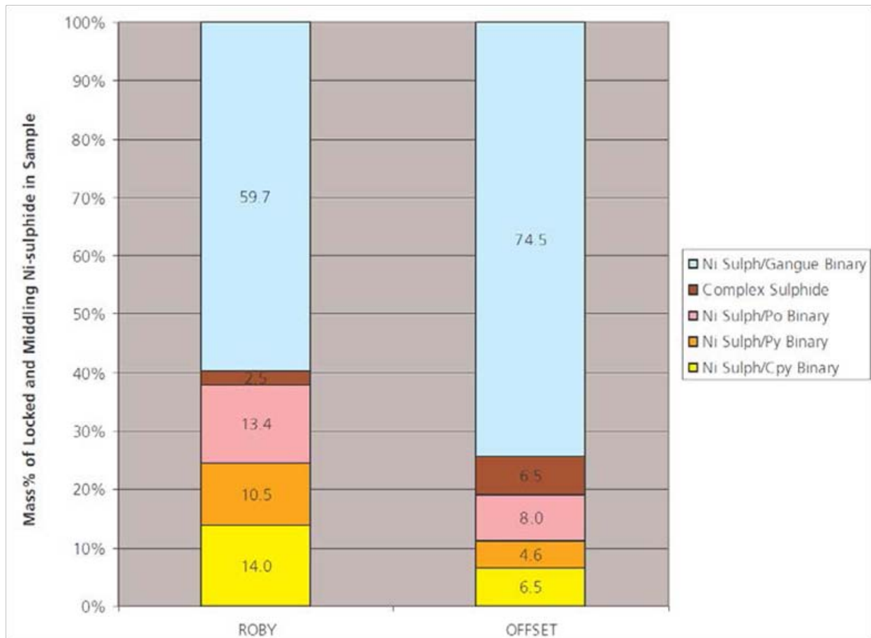
Figure 13-4: Nickel Sulphide Locking Characteristics - Source: XPS (2010)
